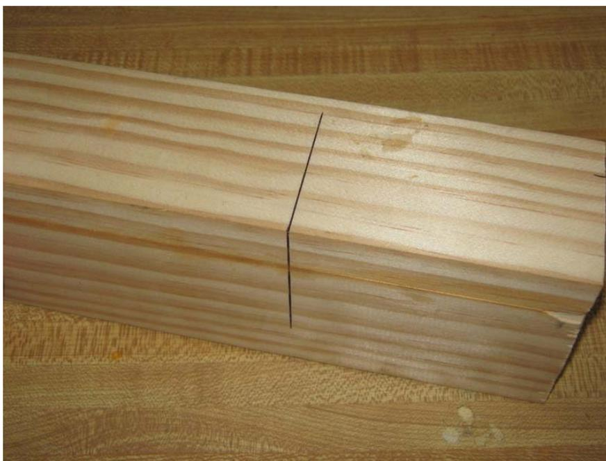
Now, make a mark on each of these lines, at the distance you measured earlier ( $1 \frac{7}{8}$ " in my case) from the apex's edge. Make another mark on the apex's edge,  $5 \frac{1}{2}$ " from the lines, and trace a diagonal between the marks.
